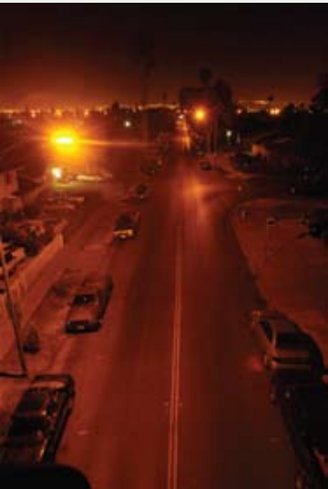
FIGURE 1. Low pressure sodium streetlights (top) were retrofitted with LED luminaires (bottom) in San Jose, CA, for 62% energy savings.
