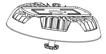
2. Remove the plastic plug by unscrewing the lock nut attached to the screw.
