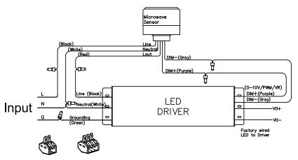
4. Connect the wires according to the wiring diagram. Wago connectors are recommended.
