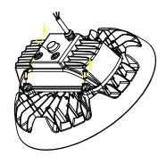
1. Detach the driver box by unscrewing the 4 screws.
