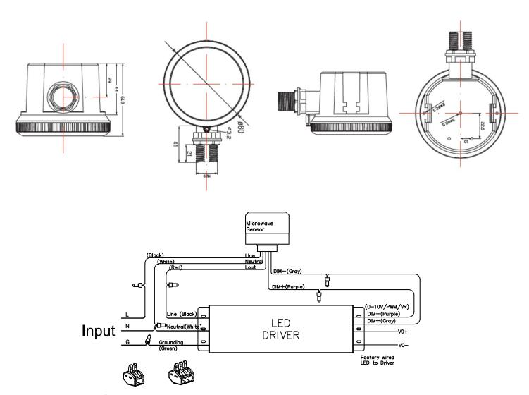
Connect the wires according to the wiring diagram. Wago connectors are recommended.
