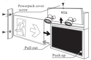
2. Knockout back of housing and push wires through the hole.
