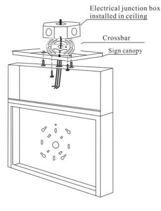
3. Make the proper supply lead connections.
