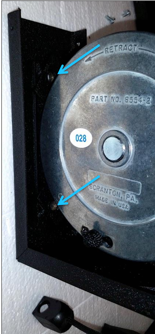
Figure 13. enclosure bracket with 2 pre-drilled holes for mounting
