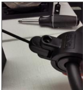
Figure 8. Top part of the hose clamp
